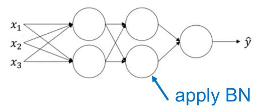
Without BN, layer 2 depends on output of layer 1 hence params of layer 1 With BN, mean and variance of  $z^{(2)}$  unchanged
